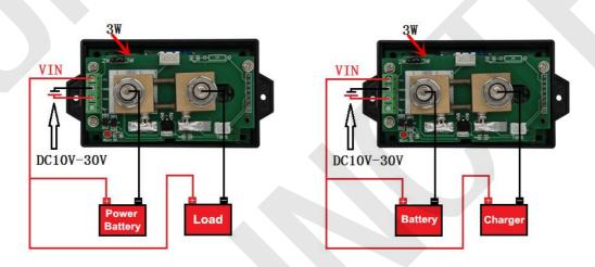
The figure above applies to batteries or circuits where the VAT4300 measures 0-400V and VAT1050, VAT1100, VAT1200, and VAT1300 to 0-100V; at this time, note that the jumper cap must be connected to 3W and need to use a 10-30V. The DC voltage supplies power to the measurement module; the wiring method on the left is suitable for the discharge measurement of the battery and the measurement of the DC circuit; the wiring method on the right is only suitable for the charge measurement of the battery.
