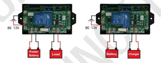
The wiring method on the left is applicable to the discharge measurement of the battery and the measurement of the DC circuit; the wiring method on the right is only applicable to the charge measurement of the battery.
