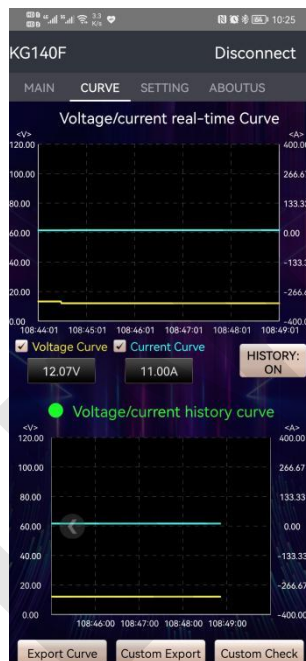
Figure 3-5-24 Voltage/current history curve
