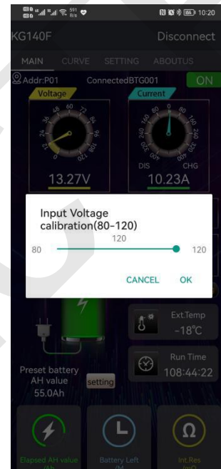
Figure 3-5-13 Input Voltage calibration
