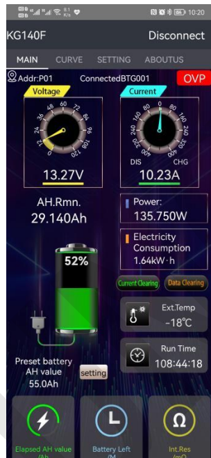
Figure 3-5-12 Over-voltage protection status
