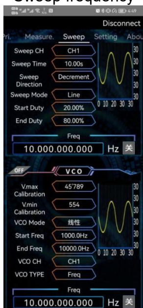
Figure 3-9-35 Voltage control frequency
