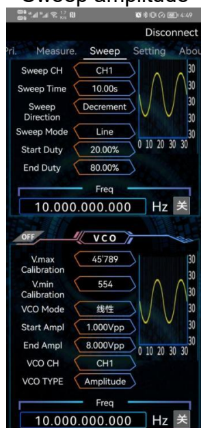
Figure 3-9-36 Voltage control amplitude
