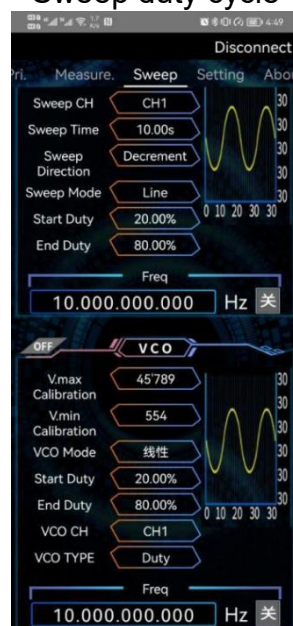
Figure 3-9-37 Voltage control duty cycle
