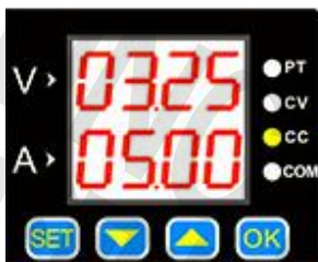
When the load current reaches the set current, the output is the set current, constant current output, and the CC indicator is on.
