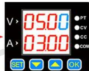
Press the SET button continuously, the flashing position will move at different positions of voltage and current.
