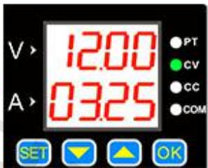
Press OK to turn the output on or off. When the load current is less than the set current, the output is constant voltage output and the CV indicator is on.
