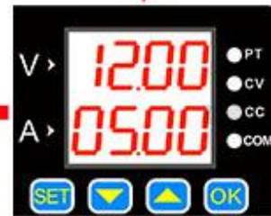
The flashing position can be changed by up and down buttons, such as adjusting 12V, 5A. Press OK to exit the adjustment state.
