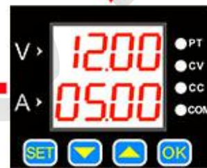
The flashing position can be changed by ▲ and ▼ buttons, such as adjusting 12V, 5A. Press OK to exit the adjustment state.
