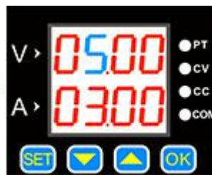
Press SET button shortly, a value flashes.
